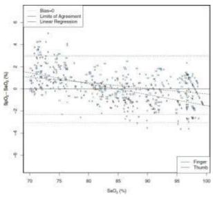
This graph shows plots of the error (Sp02 – Sa02) by Sa02 using the 3230 with a linear regression fit and upper 95% and lower 95% limits of agreement. Each sample data point is identified by subject from a clinical study in non-motion conditions.
